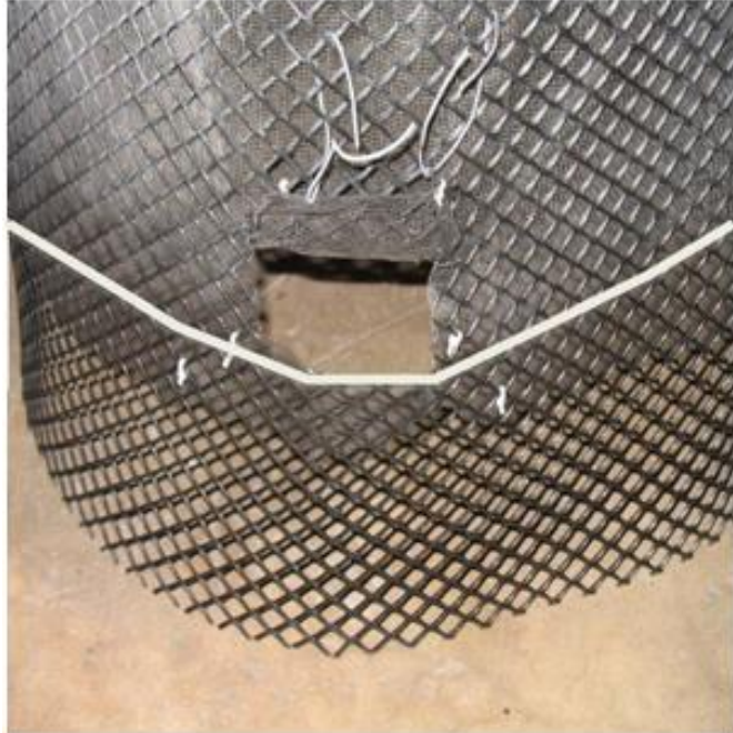
Appendix 2a: Sea turtle hatchling restraining cage design with escape door. Size: ~24 inches height by 24 inches diameter.
