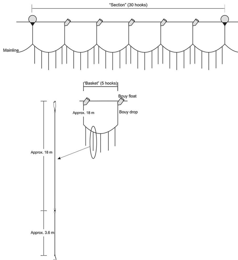
**Fig. 2.** Pelagic longline. Schematic drawing of the gear used in the pelagic bycatch experiment to compare the performance of circle and traditional J-style hooks by alternating them throughout the set.
