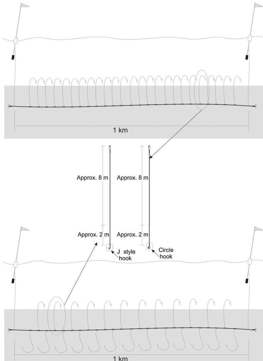
**Fig. 3.** Demersal longline. Schematic drawing of the coastal longline used off Recife, Brazil; bottom: first phase, using only J-style hooks either suspended in the water column or laying on the bottom; middle: details of the branch lines utilized in both phases; top: second phase, using alternating J-style and circle hooks both suspended in the water column.
