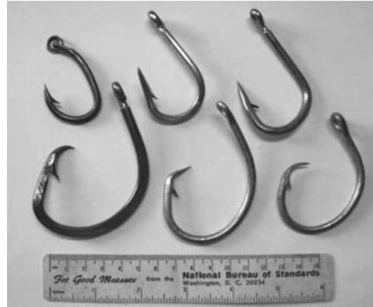
**Figure 1** Various hook types used in pelagic longline gear configurations. Clockwise from left to right, size 5/0 ringed tuna hook, size 7/0 J-style hook, size 9/0 J-style hook, size 16/0 circle hook, size 18/0 circle hook and size 20/0 circle hook. In the present study, we categorized tuna hooks with J-hooks based on the similarities in the orientation of the point relative to the shank (see text for details).
