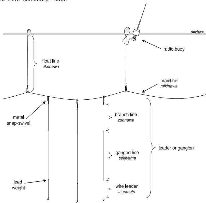
to increase visibility. In later years, a carbide lamp or battery-powered light was also attached to help monitor the movement of the gear during nighttime deployments and glass and wooden floats were replaced with aluminum floats. Float lines are stored in either plastic baskets or on spools.
