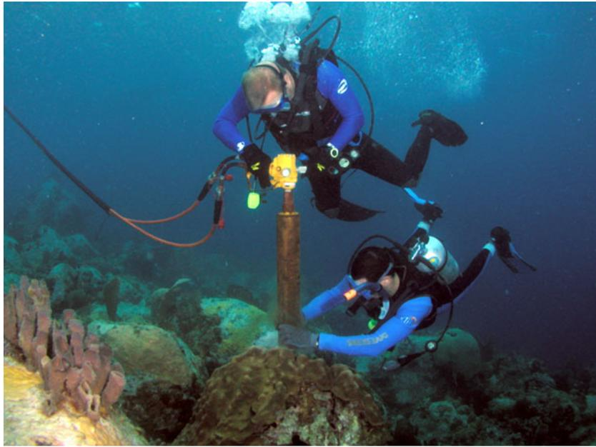
**Sclerochronology, Figure 2** Coring of a coral colony using a hydraulic drill to obtain a skeletal record of coral growth rates.
