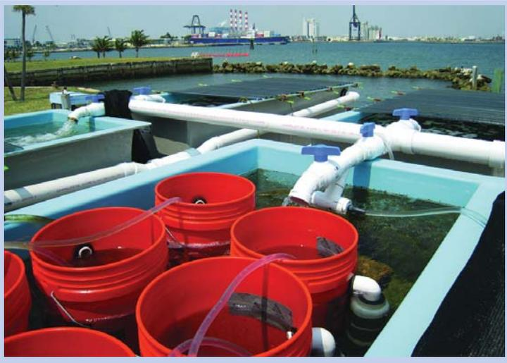
Larval collection buckets. Each orange bucket contains one colony of *P. astreoides*. White jars attached to orange buckets collect larvae as water flows out of the buckets.
